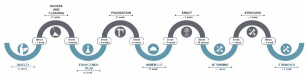
Figure 1.3 Indicative duration of construction activities at transmission line towers
