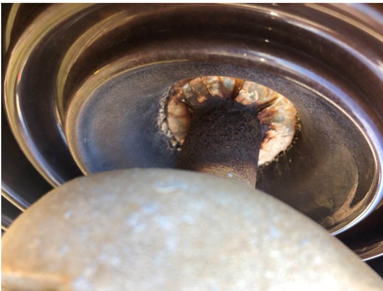
Figure 2-5 Rust on Insulator Pins
