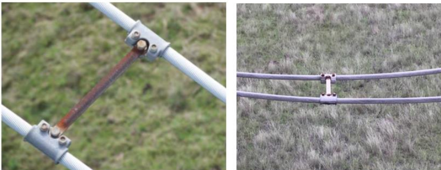
Figure 2-5 Corrosion affecting conductor fitting attachments
