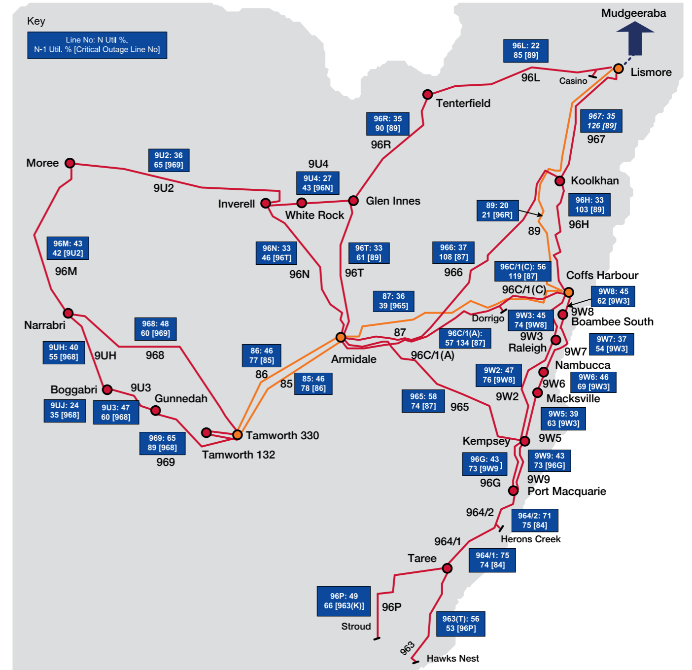
FIGURE A3.6 – TransGrid N and N-1 line utilisations – North Coast and North West 132 kV System
