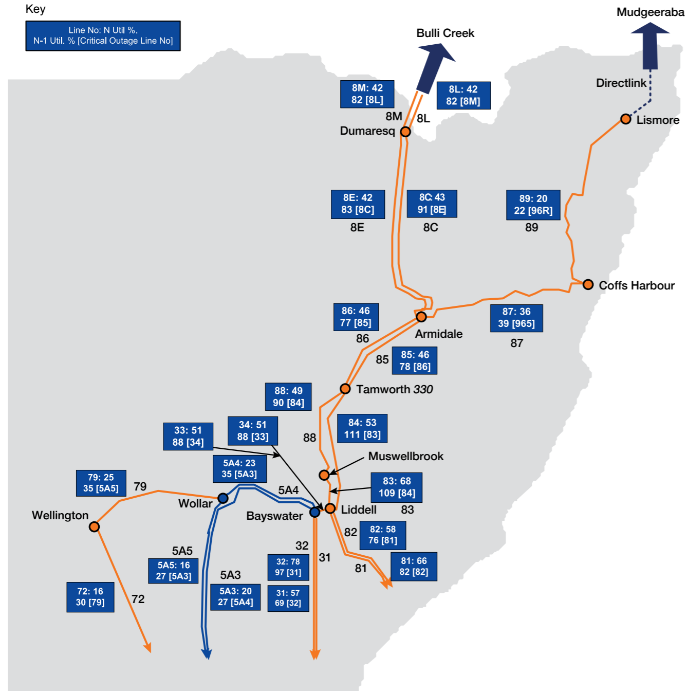
FIGURE A3.3 – TransGrid N and N-1 line utilisations – North East NSW and Hunter Valley
