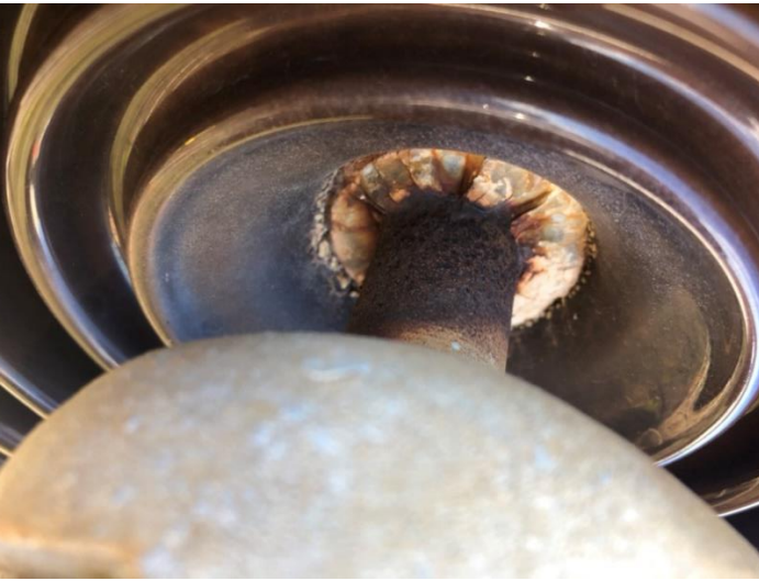
Figure 2-5 Rust on insulator pins
