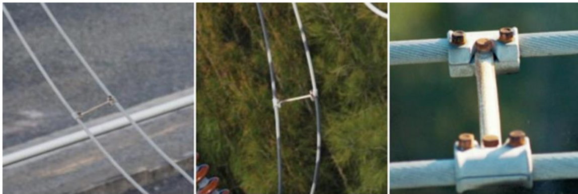
Figure 2.4 Corroded bolt and nuts of spacers
