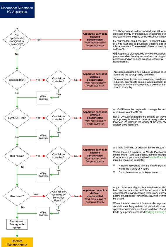
The HV apparatus is disconnected from all sources of HV electrical energy by the removal or absence of conductors and cannot be energised by electrical operating work.
