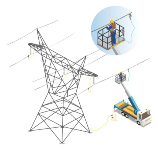
Bridging leads should be applied, to maintain a current path before a conductor is to be connected or disconnected.
