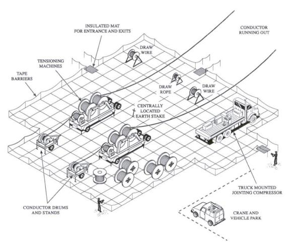
Main work sites are normally established as a bonded work area. All material and equipment associated with the running of draw wires, earth wires and conductors are bonded to the work area. Entrance to or exit from the bonded work area is normally via insulating mats, with a taped barrier defining the edges of the bonded work area.
