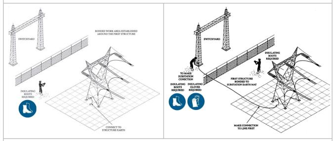
Winches, brakes and other equipment associated with the stringing operation are to be connected to the switchyard earth grid directly or via the earthing of the first structure using the process outlined above. The following options may be used:
