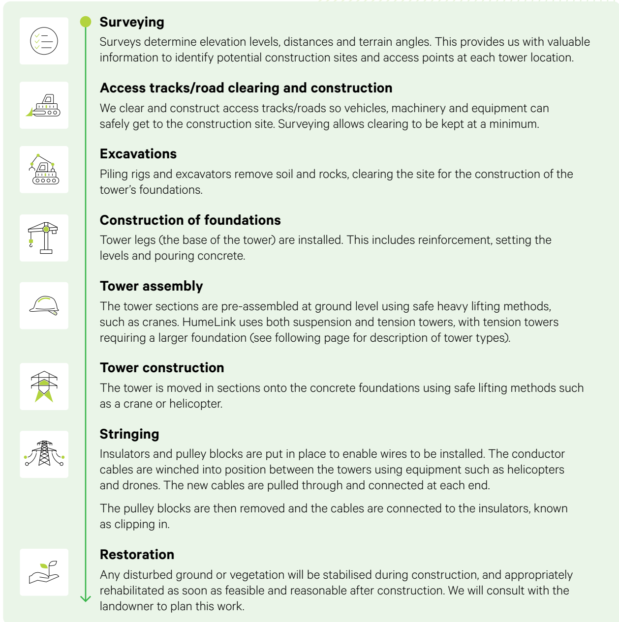
Figure 5: Transmission line construction process.
