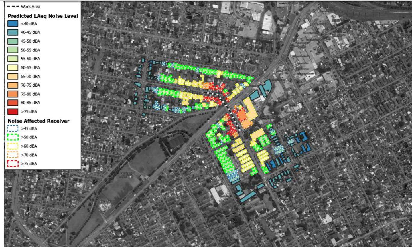
Figure 1: Extract from project OOHV CNVIS showing location at intersection Punchbowl Road and Wangee Road and noise impacted receivers.
