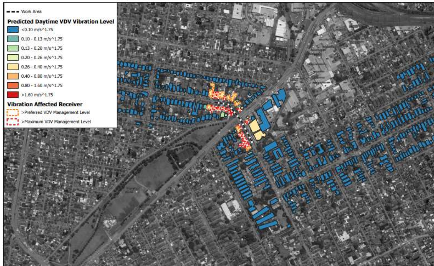
Figure 2: Extract from project OOHV CNVIS showing location at intersection Punchbowl Road and Wangee Road and vibration impacted receivers.
