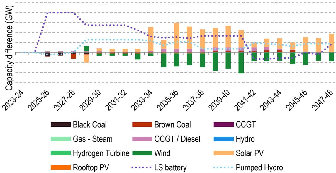
Figure 20: Difference in NEM generation forecast between Option 1A(4) and Base Case in the Progressive Change scenario (including forecast generation of Option 1A(4))
