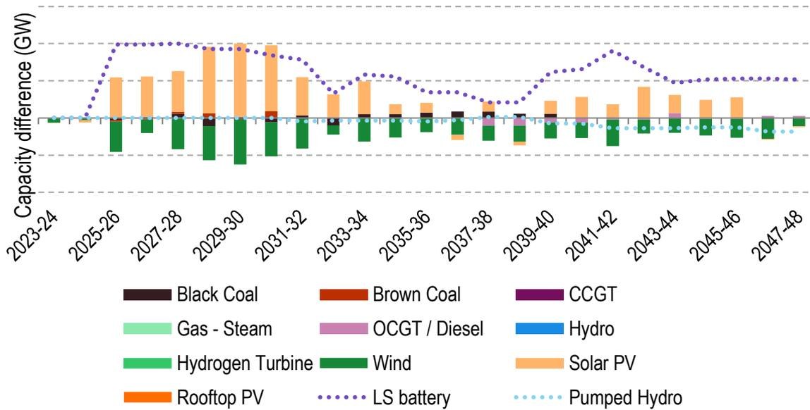
Figure 17: Difference in NEM generation forecast between Option 1A(4) and Base Case in the Step Change scenario (including forecast generation of Option 1A(4))
