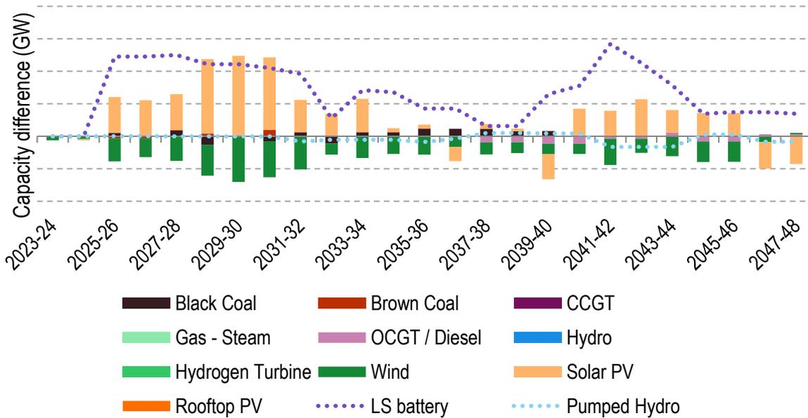
Figure 26: Difference in NEM generation forecast between Option 1A(2) and Base Case in the Step Change scenario (including forecast generation of Option 1A(2))
