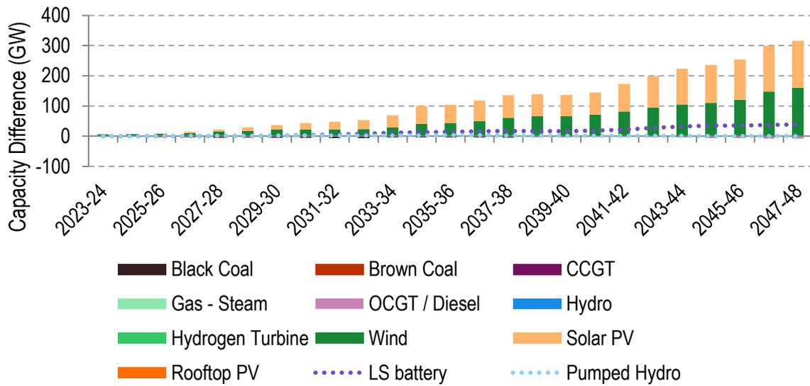
Figure 14: Difference in NEM generation forecast between the Hydrogen Superpower and Step Change scenarios in the Base case (excluding rooftop PV)
