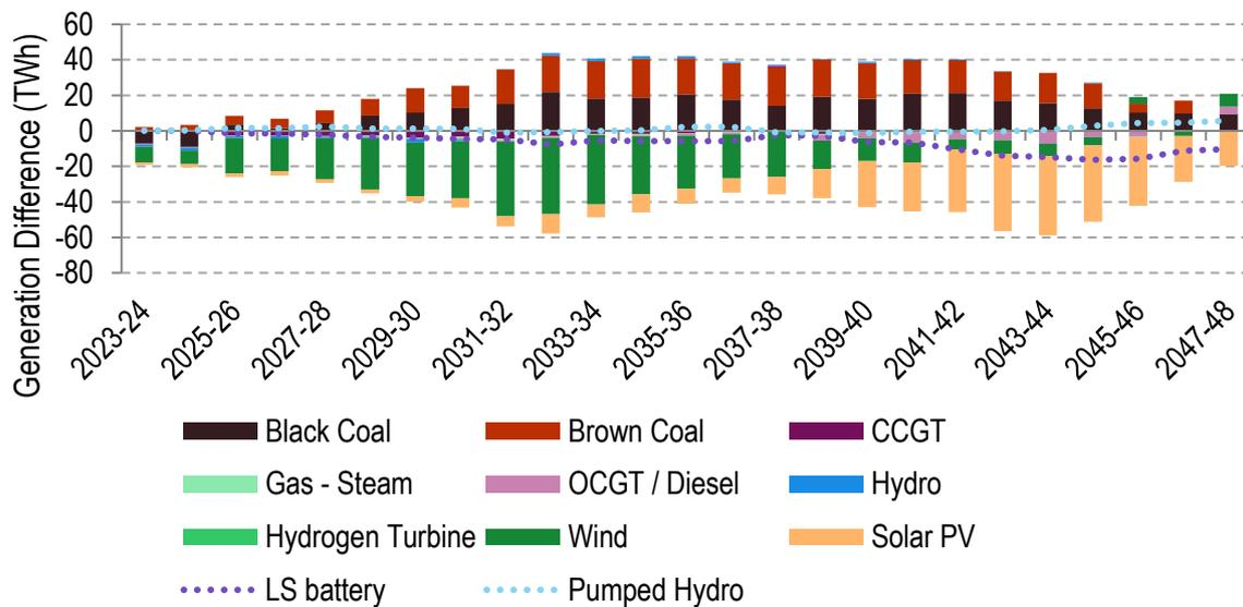
Figure 13: Difference in NEM capacity forecast between the Hydrogen Superpower and Step Change scenarios in the Base case (excluding rooftop PV)
