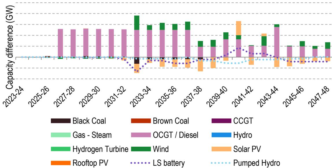
Figure 32: Difference in NEM generation forecast between Option 3 and Base Case in the Step Change scenario (including forecast generation of Option 3)
