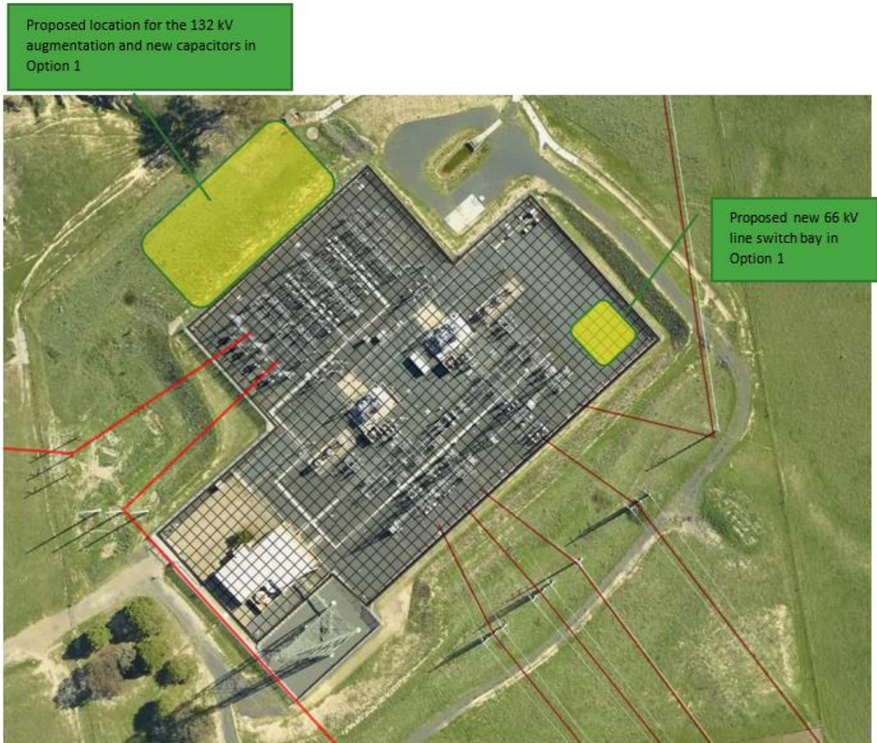
Figure 3-1 Indicative location of the proposed works at Panorama 132/66kV substation for Option 1
