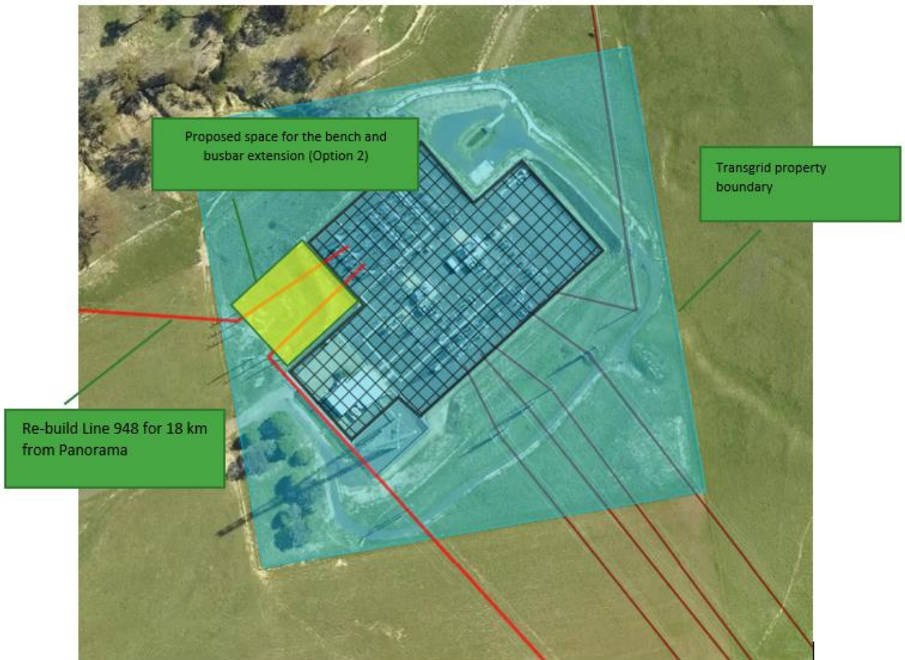
Figure 3-3 Indicative location for the proposed works at Panorama 132/66 kV substation under Option 2
