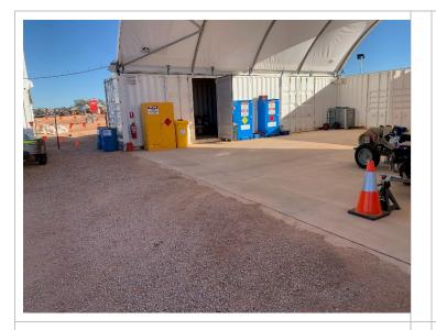
**Photo 13:** Chemical storage cabinet, spill kits and covered hardstand area Camp 6
