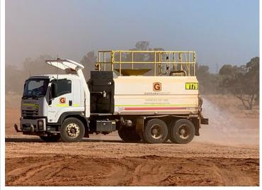
Photo 6: Water cart in operation – Buronga Substation Site
