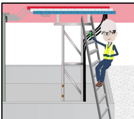
Staying at ground level in HV areas and not climbing on HV structures.
