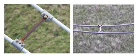
Figure 2-5 Corrosion affecting conductor fitting attachments
