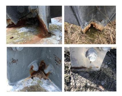
Figure 2-4 Corrosion affecting conductor spacer
