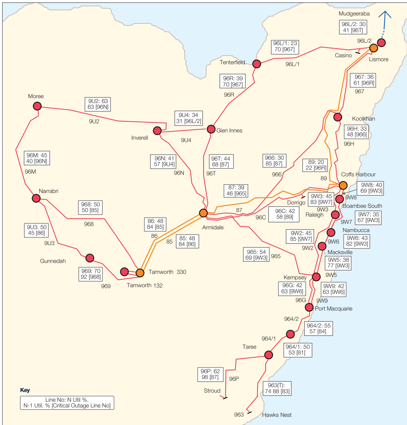
FIGURE A5.7 – TRANSGRID N AND N-1 LINE UTILISATIONS – MAP 6 – NORTH COAST AND NORTH WEST 132 kV SYSTEM
