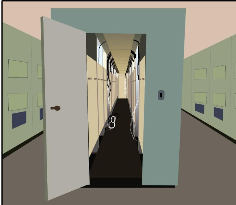
Barriers should be installed at any location where live equipment is installed in the panel. You can remove a barrier while you require access to the panel.
