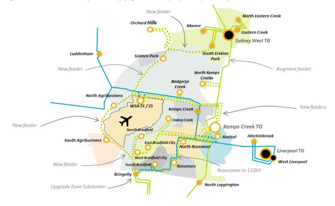
Figure 2-1 Overview of the electricity network supplying the Western Sydney Aerotropolis Priority Growth Area
