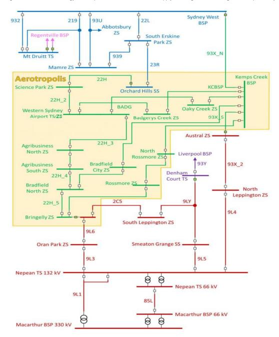
Figure 3-3 Endeavour Energy Aerotropolis Area Plan for 132 kV supply showing network configuration expected by 2035-2040
