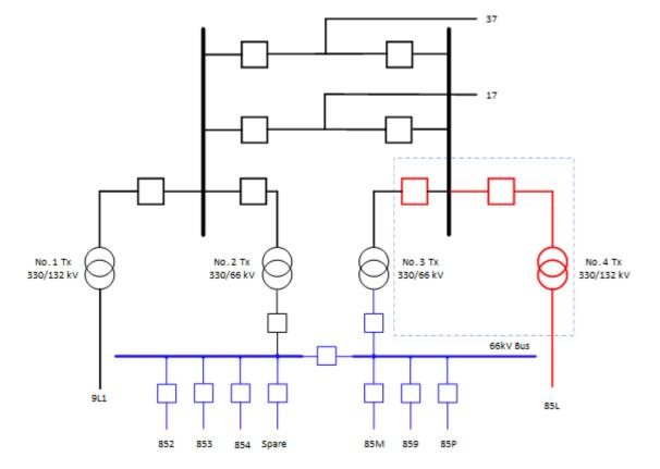
Figure 3-2 Macarthur BSP layout for connecting one new 330/132 kV transformer (for both options 1 and 2)
