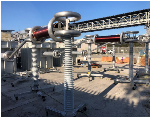
HVAC test setup for 330kV at Alexandria
