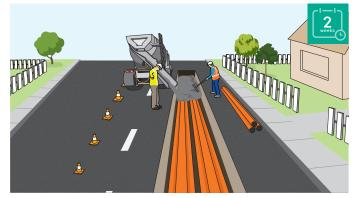
Trenching will involve digging a trench around three metres wide and installing pipes to house the cables. Work takes around two weeks near each property.
