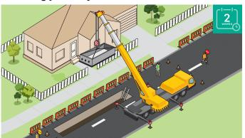
Joint bays will be installed roughly every 900m along the cable route. Work takes around two weeks at each location.
