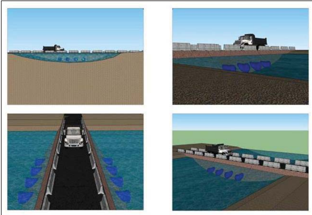
Figure 4-4: Indicative diagram of a large diameter culvert crossing used for dam crossings
