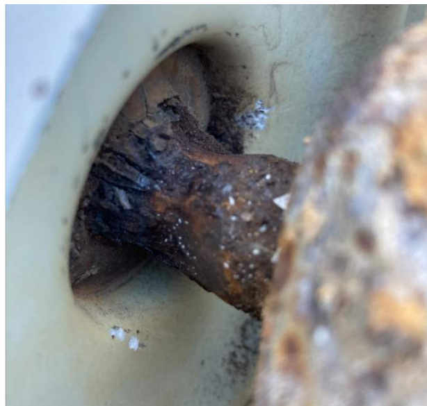
Figure 2-4 Corroded insulator pins
