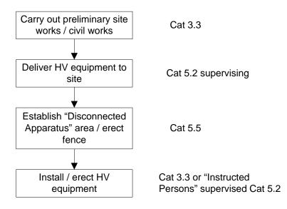
If desired, it is acceptable to erect the fence earlier in the work sequence as a safety barrier whilst the civil works are carried out (provided it is appropriately earthed). However, the "Disconnected Apparatus" signs should only be affixed once the HV equipment has been delivered.
