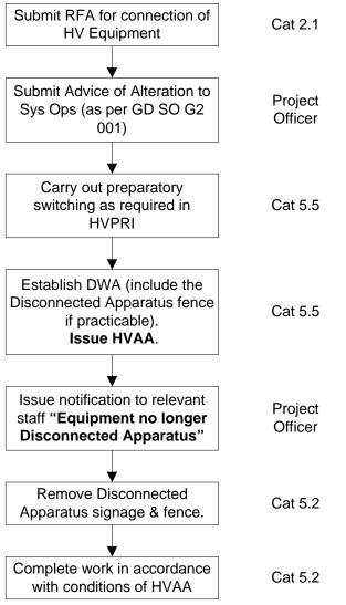
Note the requirement to establish the DWA outside the Disconnected Apparatus fence if practicable. This means that the fence can be removed under the control of the Access Authority, so that it is apparent to all staff that the equipment is always either Disconnected Apparatus or requires a HVAA for work.
