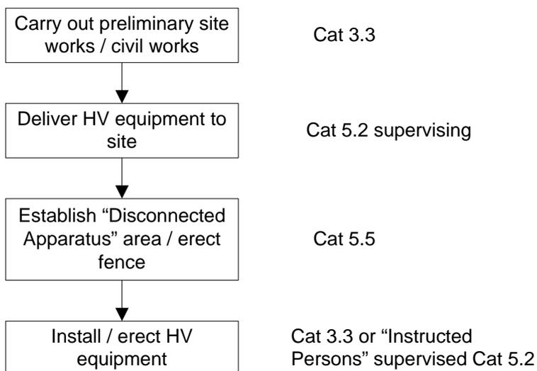
If desired, it is acceptable to erect the fence earlier in the work sequence as a safety barrier whilst the civil works are carried out (provided it is appropriately earthed). However, the “Disconnected Apparatus” signs should only be affixed once the HV equipment has been delivered.
