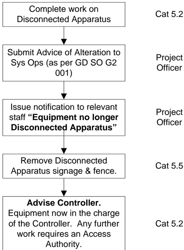
The advice to staff is extremely important, especially when a project team have been allowed full access previously and could believe the equipment to still be disconnected from the HV network.
