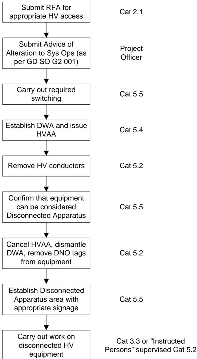
If the equipment is to be decommissioned and removed from site, then this can be carried out after the final step under the supervision of a person authorised cat 5.2, after which the fence can be removed.
