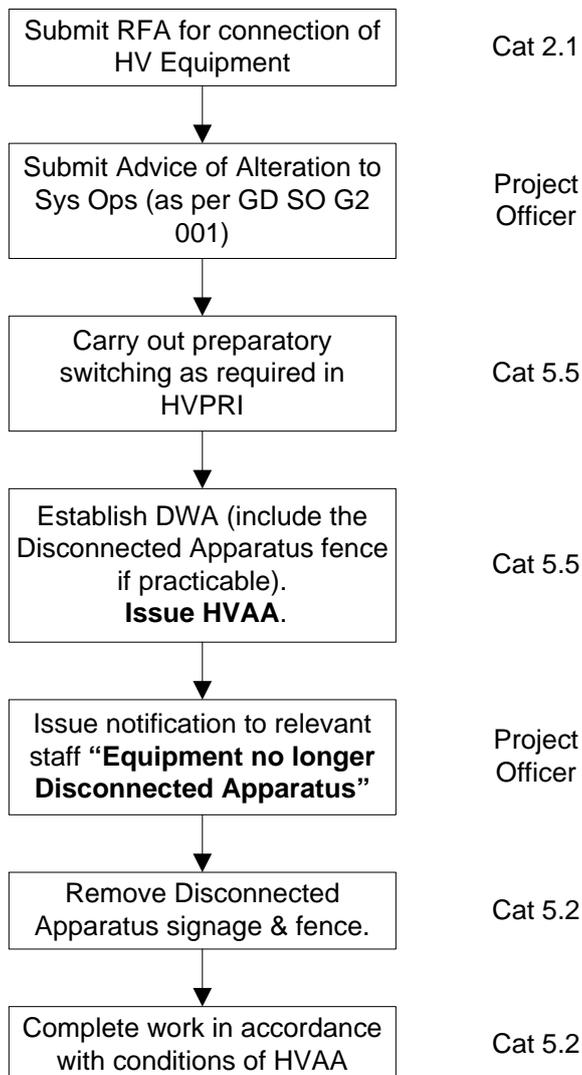
Note the requirement to establish the DWA outside the Disconnected Apparatus fence if practicable. This means that the fence can be removed under the control of the Access Authority, so that it is apparent to all staff that the equipment is always either Disconnected Apparatus or requires a HVAA for work.
